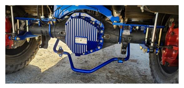
For the F-550, spacers are required on both side mounts. When reinstalling sway bar include the spacers on each side using the bolts supplied with spacer kits. Tighten bolts 25-30 Ft lbs.
